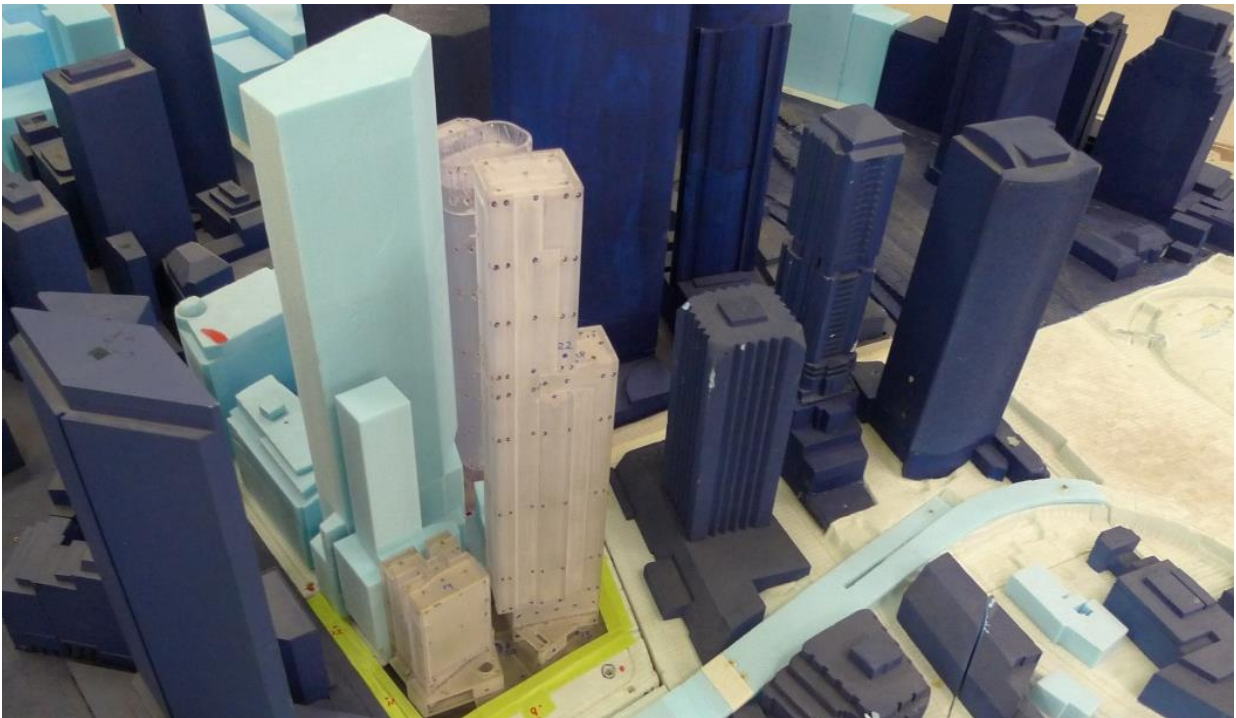
Figure 4: CPP Wind tunnel model of original LLCQ model, view from north-east
